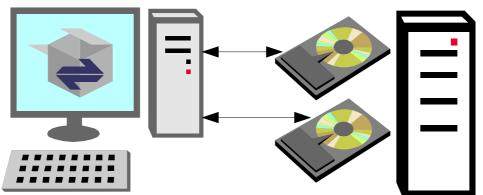
Figure 12: Automatic software distribution on a client. An opsi server provides configuration information and installable software packets.
