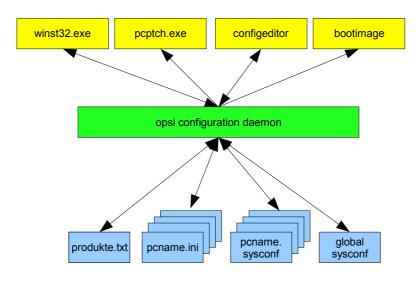
Figure 2: opsi V3 using the web service for data access
